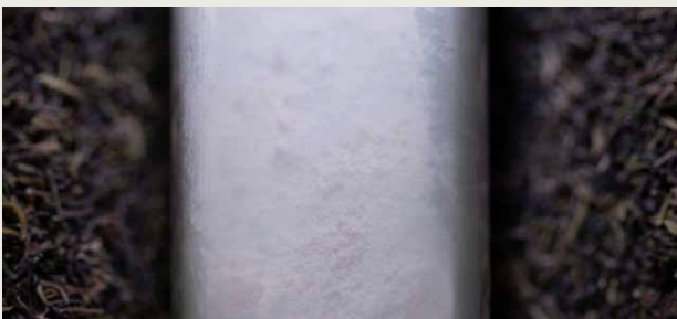
PHA powder produced from (and set in between) our farmed seaweed feedstock, Gracilaria .
